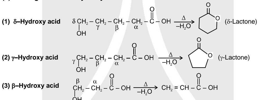
Since 4 or 8 membered rings are less stable therefore  $\beta$ -Hydroxy acids on heating produce  $\alpha, \beta$  unsaturated carboxylic acid.
