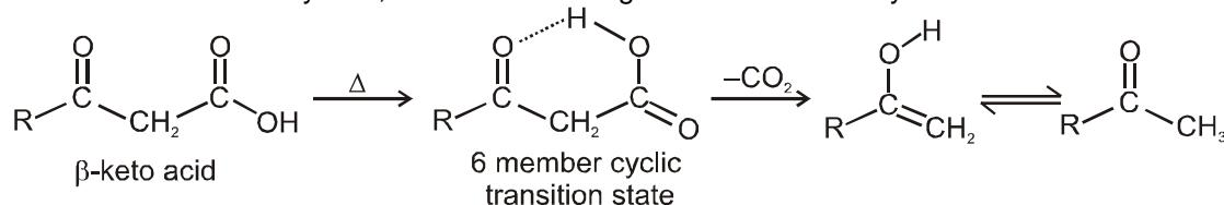
This reaction produces an enol directly and avoids an anionic intermediate. The enol then tautomerises to a methyl ketone.
